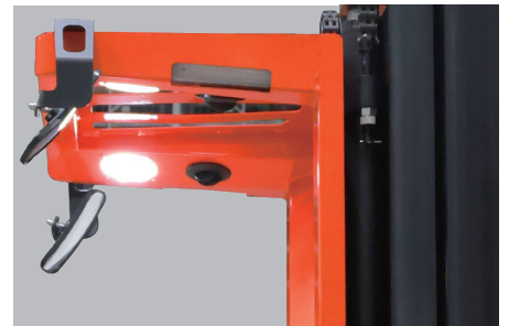
LED work lights and fan
